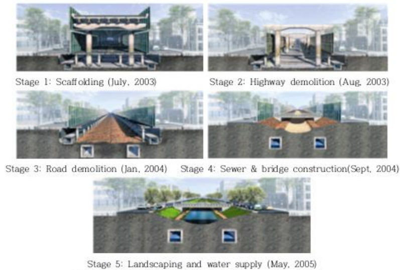
<Figure 13> Stages of the Cheonggyecheon restoration work
