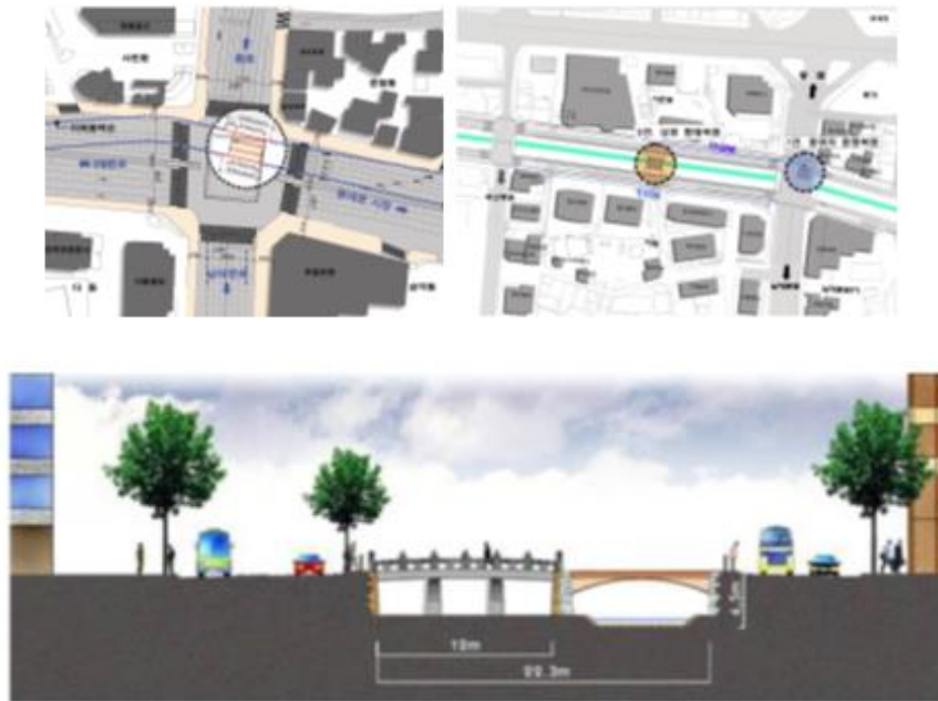
<Figure 18> Gwangtonggyo: original location, alternative location, and restored cross section 5)
